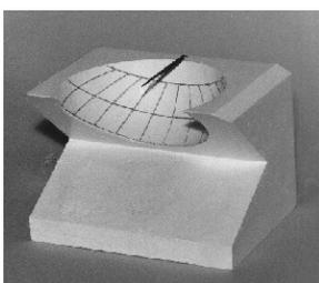
The Romans used the shadow of the end of a horizontal rod against the inside of a sphere carved out from stone. Some had several scales of time for different dates of the year. So, in fact such dials were able to tell both time and even an estimate of date. However the shadow of the whole rod on such a dial forms a line that means nothing.
