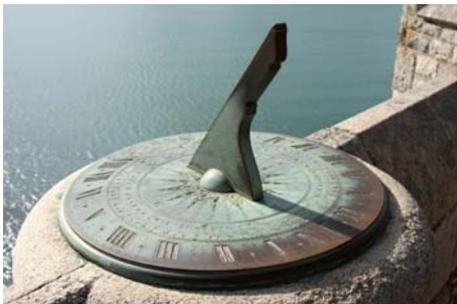
Where the gnomon might be a piece of some fairly flat thick material the shadow that is seen might over the course of a day come from either edge of the flat material, in which case each edge is called a 'style' and the time is read from the position of the shadow of the appropriate edge. Most ordinary horizontal dials use thick gnomons.
