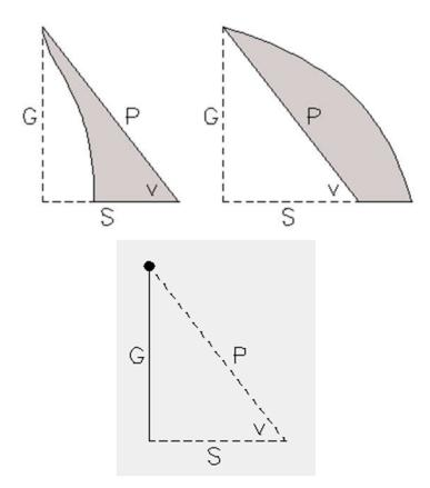
But what is the significance of G in all these drawings? A pole style can only be used to read solar time, possibly corrected for longitude. For other time systems, such as Babylonian or ancient hours, or for date lines, the shadow of a single identifiable point is required.
