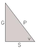
The perpendicular projection of the pole style into the dial face, where the style triangle is fixed, is the **substyle**, marked S.
